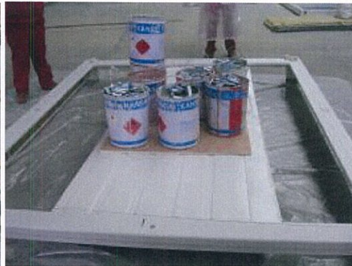
Testing during load of 572 Kg
